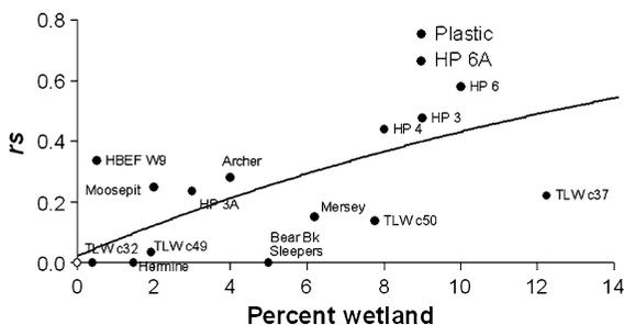
**Fig. 7** The relationship between percent wetland coverage and  $\text{SO}_4^{2-}$  response score. *Open circle* symbol represents values ( $rs = 0$  and wetlands = 0) for the Biscuit Brook, Fernow and HBEF W6 catchments
