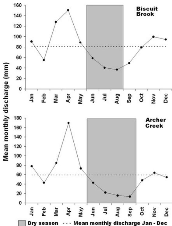
**Fig. 2** Mean monthly discharge (mm) for the Biscuit Brook (1984–2009) and Archer Creek (1995–2007) streams. *Dotted line* is the mean monthly discharge from Jan–Dec (*solid line*) and the *shaded area* indicates the dry season for each stream as defined in this study
