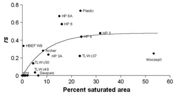
**Fig. 8** The relationship between percent saturated area and  $\text{SO}_4^{2-}$  response score. *Shaded area*  $rs$  of 0 and percent saturated area of 0 (TLW c32 and HBEF W6), 0.65 (Bear Brook), 0.87 (Fernow), 1.28 (Biscuit Brook) and 2.15 (Hermine). *Note:* no % saturated area calculated for Mersey watershed due to corrupted DEM
